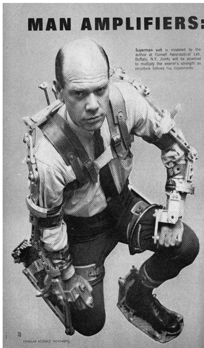
Fig. 6. Wallace Cloud wearing a superman suit created by Cornell Aeronautical Laboratory, in Wallace Cloud, "Man Amplifiers: Machines That Let You Carry a Ton," Popular Science (Nov. 1965): 70.
